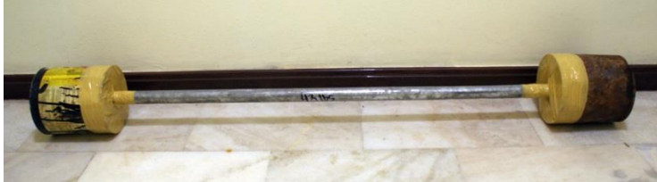
4 Liter Paint Can Barbell: 43lbs with two cans filled with concrete and a metal bar
